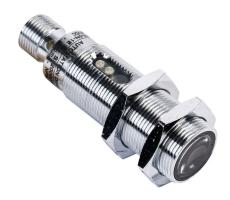
AutomationDirect photoelectric sensor, tubular, threaded, metal housing, through-beam receiver, 6m sensing distance, 10-36 VDC operating voltage, complementary light-on/dark-on, NPN, 4-wire, 4-pin M12 quick-disconnect.
