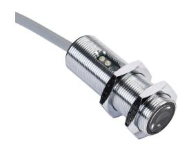
AutomationDirect photoelectric sensor, tubular, threaded, metal housing, through-beam receiver, 6m sensing distance, 10-36 VDC operating voltage, complementary light-on/dark-on, NPN, 4-wire, pigtail.
