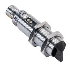
AutomationDirect photoelectric sensor, tubular, threaded, polarized retroreflective, right-angle lens, visible red, 2m sensing distance, dark-on, PNP, 3-wire, 4-pin M12 quick-disconnect.
