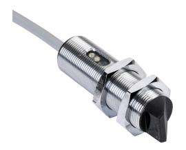
AutomationDirect photoelectric sensor, tubular, threaded, polarized retroreflective, right-angle lens, visible red light emission, 2m sensing distance, dark-on, PNP, 3-wire, pigtail.
