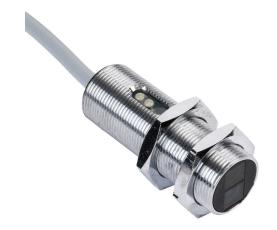
AutomationDirect photoelectric sensor, tubular, threaded, polarized retroreflective, visible red light emission, 2m sensing distance, dark-on, PNP, 3-wire, pigtail.
