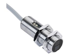
AutomationDirect photoelectric sensor, tubular, threaded, polarized retroreflective, visible red, 2m sensing distance, darkon, PNP, 3-wire, pigtail.
