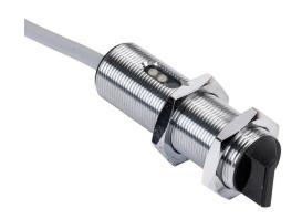
AutomationDirect photoelectric sensor, tubular, threaded, polarized retroreflective, right-angle lens, visible red, 2m sensing distance, dark-on, NPN, 3-wire, pigtail.
