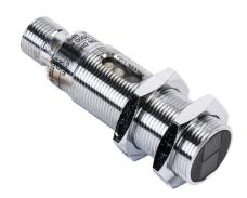
AutomationDirect photoelectric sensor, tubular, threaded, polarized retroreflective, visible red, 2m sensing distance, darkon, NPN, 3-wire, 4-pin M12 quick-disconnect.
