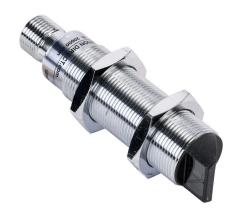
AutomationDirect photoelectric sensor, tubular, threaded, metal housing, through-beam emitter, right-angle lens, visible red light emission, 6m sensing distance, 10-36 VDC operating voltage, 3-wire, 4-pin M12 quick-disconnect.
