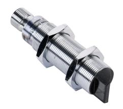
AutomationDirect photoelectric sensor, tubular, threaded, metal housing, through-beam emitter, right-angle lens, visible red, 6m sensing distance, 10-36 VDC operating voltage, 3-wire, 4-pin M12 quick-disconnect.
