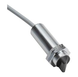
AutomationDirect photoelectric sensor, tubular, threaded, metal housing, through-beam emitter, right-angle lens, visible red, 6m sensing distance, 10-36 VDC operating voltage, 3-wire, pigtail.
