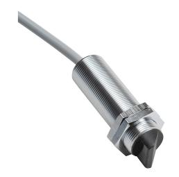
AutomationDirect photoelectric sensor, tubular, threaded, metal housing, through-beam emitter, right-angle lens, visible red light emission, 6m sensing distance, 10-36 VDC operating voltage, 3-wire, pigtail.
