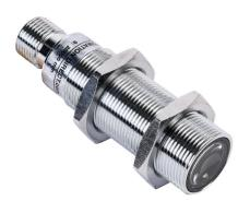
AutomationDirect photoelectric sensor, tubular, threaded, metal housing, through-beam emitter, visible red light emission, 6m sensing distance, 10-36 VDC operating voltage, 3-wire, 4-pin M12 quick-disconnect.
