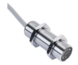
AutomationDirect photoelectric sensor, tubular, threaded, metal housing, through-beam emitter, visible red, 6m sensing distance, 10-36 VDC operating voltage, 3-wire, pigtail.
