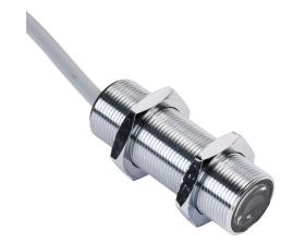
AutomationDirect photoelectric sensor, tubular, threaded, metal housing, through-beam emitter, visible red light emission, 6m sensing distance, 10-36 VDC operating voltage, 3-wire, pigtail.
