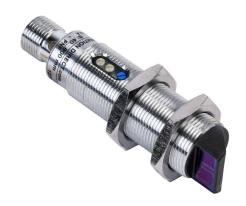
AutomationDirect photoelectric sensor, tubular, threaded, diffuse, right-angle lens, visible red, 600mm sensing distance, complementary light-on/dark-on, PNP, potentiometer, 1 kHz switching frequency, metal housing, 4-pin M12 quick-disconnect.
