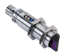
AutomationDirect photoelectric sensor, tubular, threaded, diffuse, right-angle lens, visible red light emission, 600mm sensing distance, complementary light-on/dark-on, PNP, potentiometer, 1 kHz switching frequency, metal housing, 4-pin M12 quick-disconnect.
