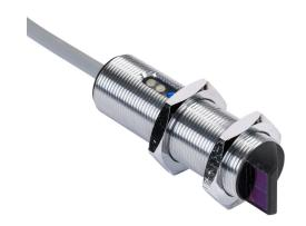
AutomationDirect photoelectric sensor, tubular, threaded, diffuse, right-angle lens, visible red, 600mm sensing distance, complementary light-on/dark-on, PNP, potentiometer, 1 kHz switching frequency, metal housing, pigtail.
