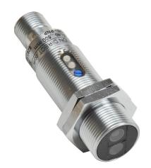
AutomationDirect photoelectric sensor, tubular, threaded, diffuse, visible red, 600mm sensing distance, complementary light-on/dark-on, PNP, potentiometer, 1 kHz switching frequency, metal housing, 4-pin M12 quick-disconnect.
