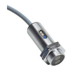
AutomationDirect photoelectric sensor, tubular, threaded, diffuse, visible red, 600mm sensing distance, complementary light-on/dark-on, PNP, potentiometer, 1 kHz switching frequency, metal housing, pigtail.
