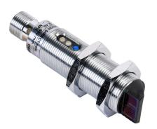
AutomationDirect photoelectric sensor, tubular, threaded, diffuse, right-angle lens, visible red, 600mm sensing distance, complementary light-on/dark-on, NPN, potentiometer, 1 kHz switching frequency, metal housing, 4-pin M12 quick-disconnect.
