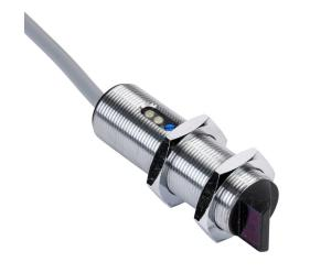
AutomationDirect photoelectric sensor, tubular, threaded, diffuse, right-angle lens, visible red, 600mm sensing distance, complementary light-on/dark-on, NPN, potentiometer, 1 kHz switching frequency, metal housing, pigtail.
