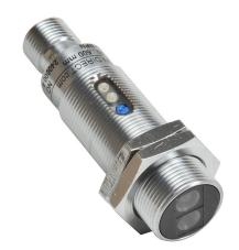
AutomationDirect photoelectric sensor, tubular, threaded, diffuse, visible red, 600mm sensing distance, complementary light-on/dark-on, NPN, potentiometer, 1 kHz switching frequency, metal housing, 4-pin M12 quick-disconnect.
