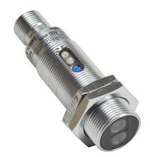
AutomationDirect photoelectric sensor, tubular, threaded, diffuse, visible red light emission, 600mm sensing distance, complementary light-on/dark-on, NPN, potentiometer, 1 kHz switching frequency, metal housing, 4-pin M12 quick-disconnect.
