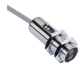
AutomationDirect photoelectric sensor, tubular, threaded, diffuse, visible red light emission, 600mm sensing distance, complementary light-on/dark-on, NPN, potentiometer, 1 kHz switching frequency, metal housing, pigtail.
