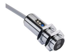
AutomationDirect photoelectric sensor, tubular, threaded, diffuse, visible red, 600mm sensing distance, complementary light-on/dark-on, NPN, potentiometer, 1 kHz switching frequency, metal housing, pigtail.
