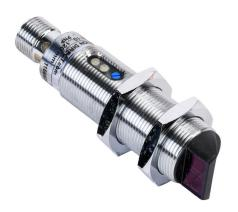
AutomationDirect photoelectric sensor, tubular, threaded, metal, diffuse with background suppression, right-angle lens, 10-120mm sensing distance, light-on, PNP, potentiometer, 500 Hz switching frequency, 4-pin M12 quick-disconnect.
