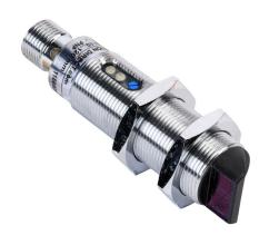
AutomationDirect photoelectric sensor, tubular, threaded, metal, diffuse with background suppression, right-angle lens, 10-120mm sensing distance, light-on, PNP, potentiometer, 500 Hz switching frequency, 4-pin M12 quick-disconnect.
