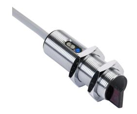
AutomationDirect photoelectric sensor, tubular, threaded, metal, diffuse with background suppression, right-angle lens, 10-120mm sensing distance, light-on, PNP, potentiometer, 500 Hz switching frequency, 6.5ft/2m cable length, pigtail.
