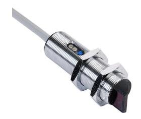
AutomationDirect photoelectric sensor, tubular, threaded, metal, diffuse with background suppression, right-angle lens, 10-120mm sensing distance, light-on, PNP, potentiometer, 500 Hz switching frequency, 6.5ft/2m cable length, pigtail.
