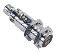
AutomationDirect photoelectric sensor, tubular, threaded, metal, diffuse with background suppression, 10-120mm sensing distance, light-on, PNP, potentiometer, 500 Hz switching frequency, 4-pin M12 quick-disconnect.
