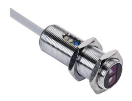
AutomationDirect photoelectric sensor, tubular, threaded, metal, diffuse with background suppression, 10-120mm sensing distance, light-on, PNP, potentiometer, 500 Hz switching frequency, 6.5ft/2m cable length, pigtail.
