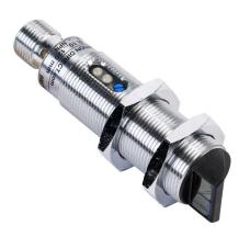
AutomationDirect photoelectric sensor, tubular, threaded, metal, diffuse with background suppression, right-angle lens, 10-120mm sensing distance, light-on, NPN, potentiometer, 500 Hz switching frequency, 4-pin M12 quick-disconnect.
