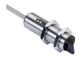
AutomationDirect photoelectric sensor, tubular, threaded, metal, diffuse with background suppression, right-angle lens, 10-120mm sensing distance, light-on, NPN, potentiometer, 500 Hz switching frequency, 6.5ft/2m cable length, pigtail.
