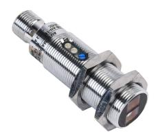
AutomationDirect photoelectric sensor, tubular, threaded, metal, diffuse with background suppression, 10-120mm sensing distance, light-on, NPN, potentiometer, 500 Hz switching frequency, 4-pin M12 quick-disconnect.
