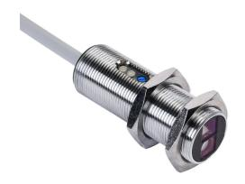
AutomationDirect photoelectric sensor, tubular, threaded, metal, diffuse with background suppression, 10-120mm sensing distance, light-on, NPN, potentiometer, 500 Hz switching frequency, 6.5ft/2m cable length, pigtail.
