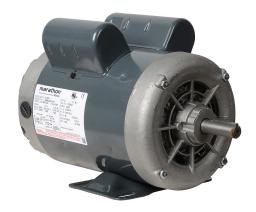
Marathon standard efficiency AC induction motor, general purpose, 2hp, 1-phase, 115/230 VAC, suitable for 208 VAC at 60 Hz, 3600rpm, ODP, NEMA 56 frame, rolled steel, rigid base mount.
