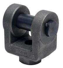
Peninsular rod clevis, 1-1/2-12 UNF thread, steel. For use with 2in rod hydraulic NFPA cylinders. 1-3/4in clevis pin included.
