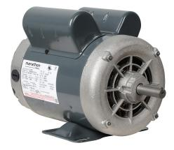
Marathon standard efficiency AC induction motor, general purpose, 1hp, 1-phase, 115/230 VAC, suitable for 208 VAC at 60 Hz, 3600rpm, ODP, NEMA 56 frame, rolled steel, rigid base mount.
