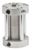
NITRA pneumatic cylinder, compact, 1-1/16in bore, 1/2in rod diameter, 2in stroke, double acting, counter-bored holes mount.
