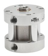
NITRA pneumatic cylinder, compact, 1-1/16in bore, 1/2in rod diameter, 1in stroke, double acting, counter-bored holes mount.
