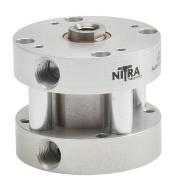
NITRA pneumatic cylinder, compact, 1-1/16in bore, 1/2in rod diameter, 3/4in stroke, double acting, counter-bored holes mount.
