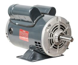
Marathon standard efficiency AC induction motor, general purpose, 1/2hp, 1-phase, 115/230 VAC, suitable for 208 VAC at 60 Hz, 1800rpm, ODP, 56 frame, rolled steel, rigid base mount.
