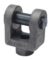
Peninsular rod clevis, 1-1/4-12 UNF thread, steel. For use with 1-3/4in rod hydraulic NFPA cylinders. 1-3/8in clevis pin included.
