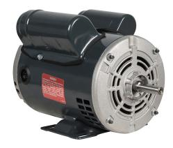
Marathon premium efficiency AC induction motor, general purpose, 1/4hp, 1-phase, 115/230 VAC, suitable for 208 VAC at 60 Hz, 1800rpm, ODP, NEMA 48 frame, rolled steel, rigid base mount.
