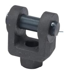
Peninsular rod clevis, 1-14 UNS thread, steel. For use with 1-3/8in rod hydraulic NFPA cylinders. 1in clevis pin included.
