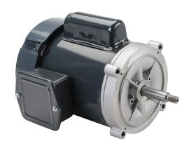
Marathon standard efficiency AC induction motor, centrifugal jet pump, 1/3hp, 1-phase, 115/230 VAC, 3600rpm, TEFC, NEMA 56J frame, rolled steel, C-face mount.
