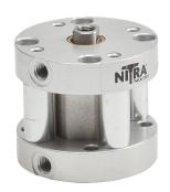
NITRA pneumatic cylinder, compact, 3/4in bore, 5/16in rod diameter, 3/4in stroke, double acting, counter-bored holes mount.
