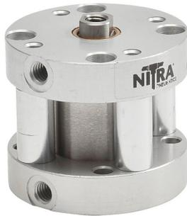
NITRA pneumatic cylinder, compact, 3/4in bore, 5/16in rod diameter, 3/4in stroke, double acting, counter-bored holes mount.
