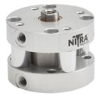
NITRA pneumatic cylinder, compact, 3/4in bore, 5/16in rod diameter, 1/2in stroke, double acting, counter-bored holes mount.
