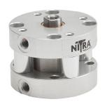
NITRA pneumatic cylinder, compact, 3/4in bore, 5/16in rod diameter, 1/2in stroke, double acting, counter-bored holes mount.
