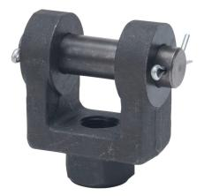
Peninsular rod clevis, 3/4-16 UNF thread, steel. For use with 1in rod hydraulic NFPA cylinders. 3/4in clevis pin included.
