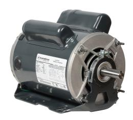
Marathon standard efficiency AC induction motor, fan and blower, 2hp, 1-phase, 115/208-230 VAC, 3600rpm, ODP, 56H frame, rolled steel, resilient base mount.
