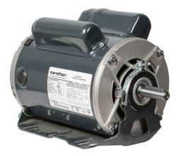
Marathon standard efficiency AC induction motor, fan and blower, 1-1/2hp, 1-phase, 115/208-230 VAC, 1800rpm, ODP, NEMA 56H frame, rolled steel, resilient base mount.
