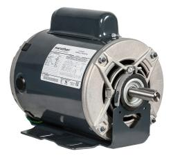
Marathon standard efficiency AC induction motor, fan and blower, 1hp, 1-phase, 115/208-230 VAC, 1800rpm, ODP, NEMA 56 frame, rolled steel, resilient base mount.
