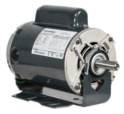
Marathon standard efficiency AC induction motor, fan and blower, 3/4hp, 1-phase, 115/208-230 VAC, 3600rpm, ODP, NEMA 56 frame, rolled steel, resilient base mount.
