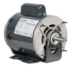
Marathon standard efficiency AC induction motor, fan and blower, 1/2hp, 1-phase, 115/208-230 VAC, 1800rpm, ODP, NEMA 56 frame, rolled steel, resilient base mount.
