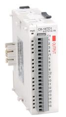
CLICK discrete output module, 16-point, 5-27 VDC, sinking, 2 isolated common(s), 8 point(s) per common, 0.1A/point. Removable terminal block included.
