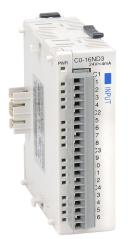
CLICK discrete input module, 16-point, 24 VDC, sinking/sourcing, 4 isolated common(s), 4 point(s) per common. Removable terminal block included.
