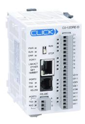
CLICK Ethernet Analog PLC, 24 VDC required, Ethernet and serial ports, Discrete Input: 4-point, DC, Analog Input: 2-channel, current/voltage, Discrete Output: 4-point, relay, Analog Output: 2-channel, current/voltage.
