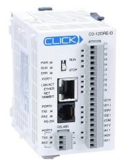
CLICK Ethernet Analog PLC, 24 VDC required, Ethernet and serial ports, Discrete Input: 4-point, DC, Analog Input: 2-channel, current/voltage, Discrete Output: 4-point, relay, Analog Output: 2-channel, current/voltage.
