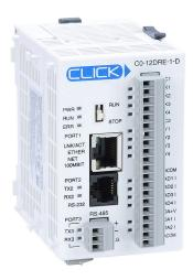
CLICK Ethernet Analog PLC, 24 VDC required, Ethernet and serial ports, Discrete Input: 4-point, DC, Analog Input: 4-channel, current, Discrete Output: 4-point, relay, Analog Output: 2-channel, current.
