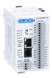
CLICK Ethernet Analog PLC, 24 VDC required, Ethernet and serial ports, Discrete Input: 4-point, DC, Analog Input: 4-channel, current, Discrete Output: 4-point, relay, Analog Output: 2-channel, current.
